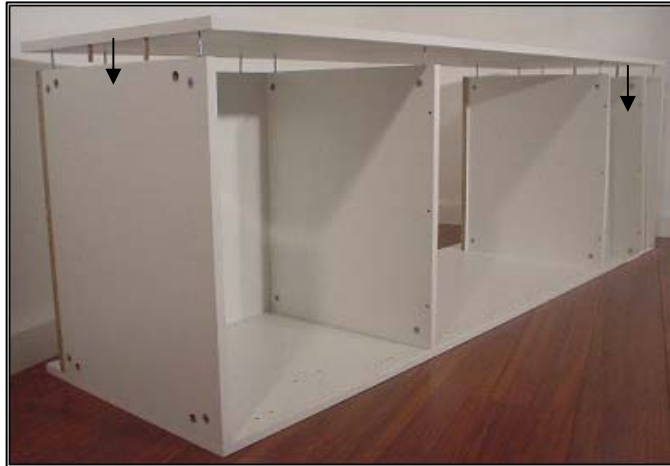
8. Fit remaining End Panel
